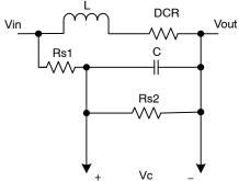
Figure 4. Inductor DCR Current Sensing Circuit
