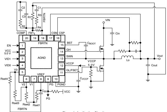
Figure 2. Application Circuit
