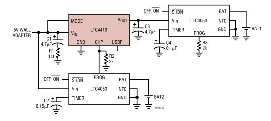
Figure 2. Priority Dual Battery Charging with Wall Adapter
