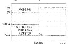
CHP Current with  $I_{LOAD}$  Step
