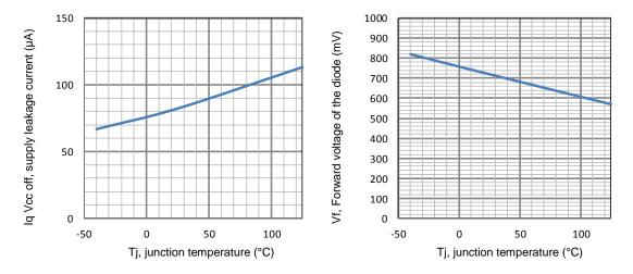
Figure 5 – Iq Vcc off (µA) Vs Tj (°C)
