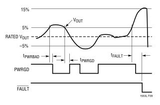
Figure 9. PWRGD and FAULT
