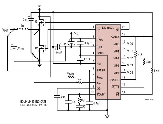
Figure 10. LTC1553L Layout Diagram
