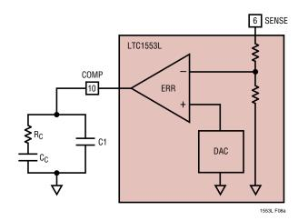
Figure 8a. Compensation Pin Hook-Up
