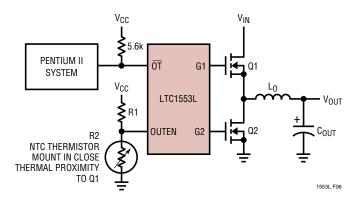
Figure 6. OUTEN Pin as a Thermistor Input
