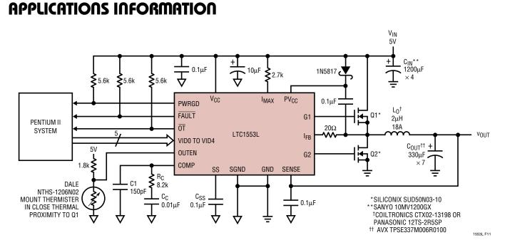
Figure 11. Single Supply LTC1553L 5V to 1.8V-3.5V Application with Thermal Monitor
