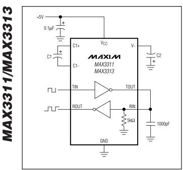
Figure 2. Loopback Test Circuit
