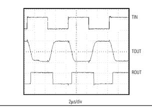
Figure 4. Loopback Test Results at 250kbps
