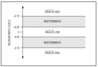
Figure 5. Receiver Positive/Negative Thresholds for INVALID
