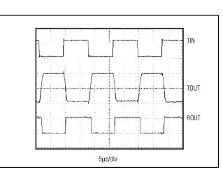
Figure 3. Loopback Test Results at 120kbps
