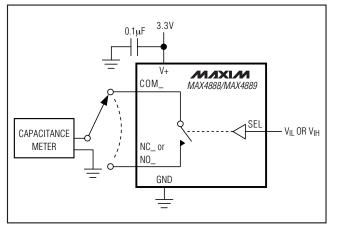
Figure 4. Channel Off-/On-Capacitance
