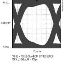
(V+ = 3.3V, f = 1.25GHz, 600mVp.p PRBS SIGNAL, R<sub>S</sub> = R<sub>L</sub> = 50Ω)<sup>†</sup> V<sub>COM\_+</sub> 50mV/div
