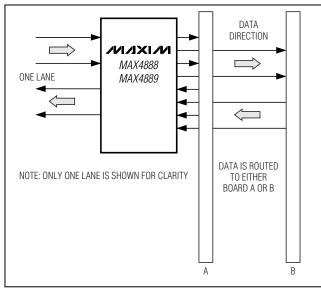
Figure 5. The MAX4888/MAX4889 Used as a Single-Lane Switch
