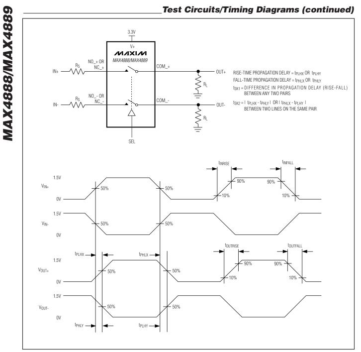
Figure 2. Propagation Delay and Output Skew
