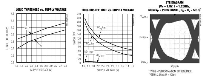
EYE DIAGRAM (V+ = 2.5V, f = 1.25GHz, 600mVp.p PRBS SIGNAL, Rs = RL = 50 $\Omega$ )<sup>+</sup>
