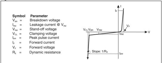
Table 2. Electrical characteristics - values ( $T_{amb} = 25 \, ^{\circ}C$ )
