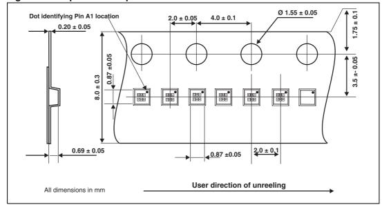
Figure 20. Tape and reel specifications
