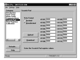
The Scratch Pad category can be used to read or write to the Scratch Pad memory locations (41101-41116). The Scratch Pad locations can be used to store user information.
