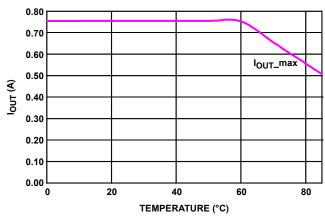
FIGURE 1. OUTPUT CURRENT DERATING
