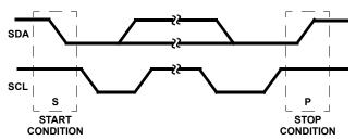
FIGURE 3. START AND STOP WAVEFORMS
