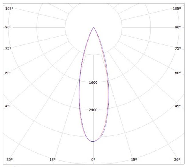
cd/klm \_\_\_\_\_\_ C0 - C180 \_\_\_\_\_ C90 - C270
