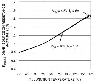
Figure 6. On-Resistance Variation with Temperature
