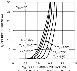
Figure 9. Diode Forward Voltage vs. Current
