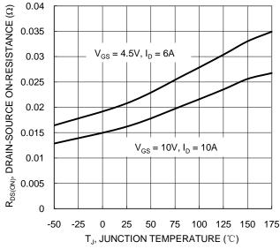
Figure 7. On-Resistance Variation with Temperature
