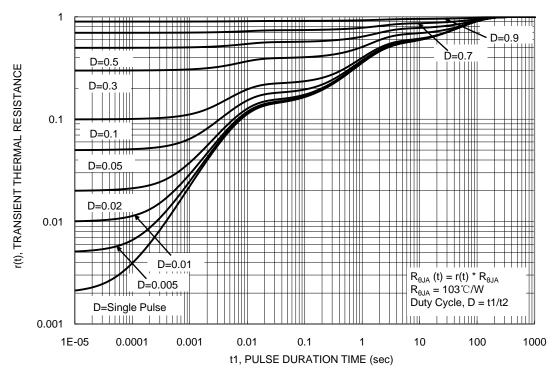
Figure 13. Transient Thermal Resistance
