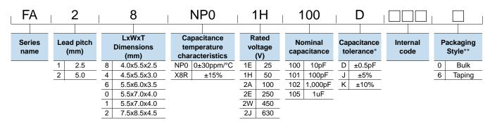
$<sup>^{\</sup>ast}$  Applicable capacitance range: Max. 10 pF for D, over 10 pF for J and K.
