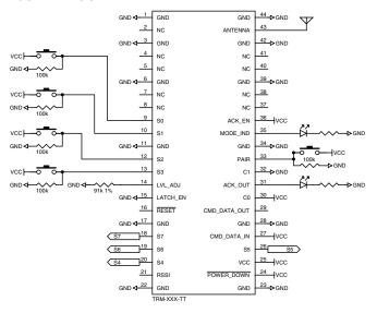
Hardware configuration with 4 inputs and 4 outputs
