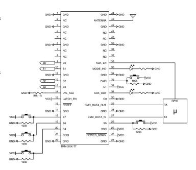
Software configuration with 4 inputs, 4 outputs and an external microcontroller
