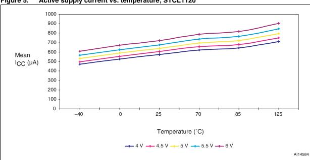
Active supply current vs. temperature, STCL1120 Figure 5.
