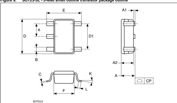
Figure 9. SOT23-5L - 5-lead small outline transistor package outline
