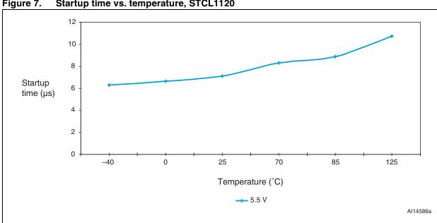
Figure 7. Startup time vs. temperature, STCL1120
