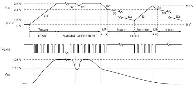
Figure 3. Voltage on Start Capacitor ( $V_{GS}$ ), the Gate ( $V_{GATE}$ ), and in the Feedback Loop ( $V_{FB}$ ), During Startup, Normal and Fault Conditions
