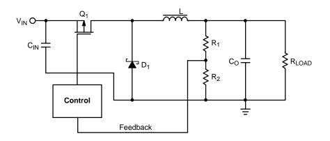
Figure 4. Buck Regulator Block Diagram
