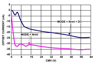
FIGURE 47. PRIMARY V<sub>SHUNT</sub> OFFSET CURRENT vs COMMON-MODE **VOLTAGE**
