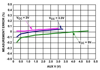
FIGURE 35. AUXILIARY V<sub>BUS</sub> MEASUREMENT ERROR vs INPUT
