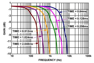
FIGURE 27. AUXILIARY  $V_{\mbox{\footnotesize{BUS}}}$  BANDWIDTH vs ADC TIMING
