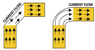
FIGURE 86. USE ARCS AND 45° TRACES TO SAFELY ROUTE TRACES WITH LARGE CURRENT FLOWS
