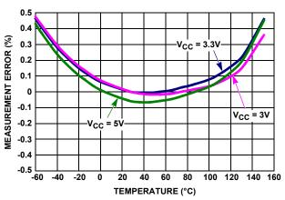
FIGURE 16. PRIMARY V<sub>SHUNT</sub> MEASUREMENT ERROR vs **TEMPERATURE**
