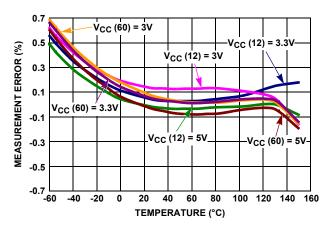
FIGURE 26. PRIMARY  $V_{\mbox{\scriptsize BUS}}$  MEASUREMENT ERROR vs TEMPERATURE
