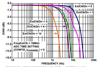
FIGURE 79. MEASUREMENT BANDWIDTH vs EXTERNAL CLK **FREQUENCY**
