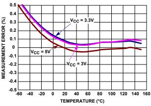
FIGURE 36. AUXILIARY V<sub>BUS</sub> MEASUREMENT ERROR vs **TEMPERATURE**
