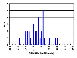
FIGURE 7. PRIMARY V<sub>SHUNT</sub> CMRR, CMV = (0V TO 60V)
