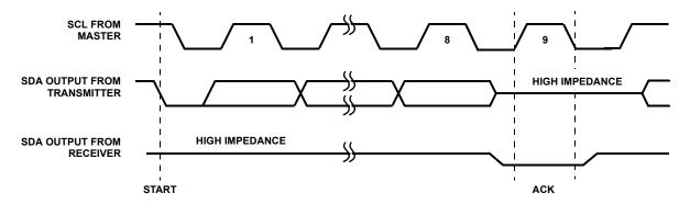
FIGURE 71. ACKNOWLEDGE RESPONSE FROM RECEIVER
