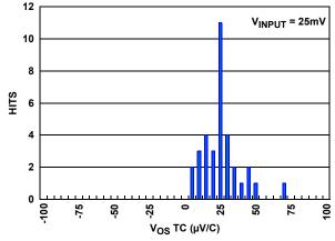
FIGURE 21. PRIMARY  $V_{BUS}$   $V_{OS}$  TC
