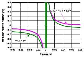
FIGURE 15. PRIMARY V<sub>SHUNT</sub> MEASUREMENT ERROR vs INPUT
