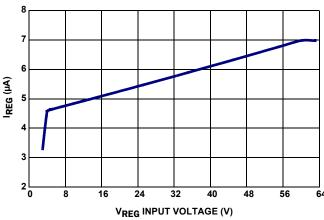
FIGURE 53.  $V_{REG}$  INPUT CURRENT vs INPUT VOLTAGE
