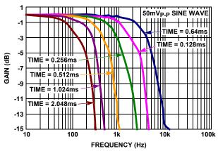
FIGURE 17. PRIMARY V<sub>SHUNT</sub> BANDWIDTH vs ADC TIMING
