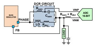
FIGURE 92. SIMPLIFIED CIRCUIT EXAMPLE OF A DCR
