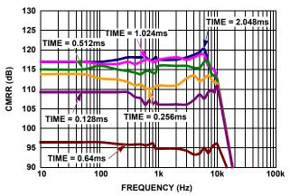
FIGURE 10. PRIMARY  $V_{SHUNT}$  AC CMRR vs FREQUENCY
