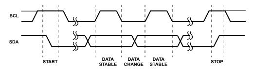
FIGURE 70. VALID DATA CHANGES, START AND STOP CONDITIONS
