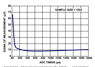
FIGURE 59. PRIMARY SHUNT STABILITY: STDEV vs ACQUISITION TIME
