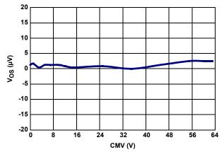
FIGURE 9. PRIMARY  $V_{SHUNT} V_{OS}$  vs CMV
