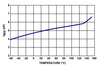
FIGURE 54.  $V_{\mbox{\scriptsize REG}}$  INPUT CURRENT vs TEMPERATURE
