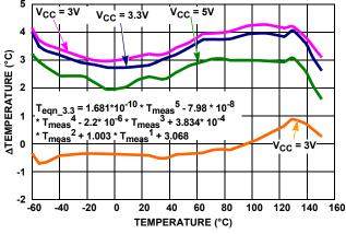
FIGURE 55. INTERNAL TEMPERATURE SENSOR ACCURACY
