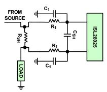
FIGURE 76. SIMPLIFIED FILTER DESIGN TO IMPROVE NOISE
