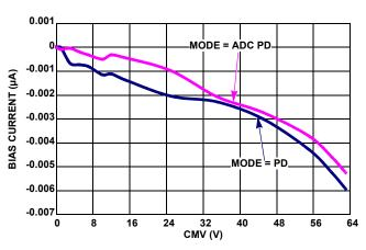
FIGURE 46. PRIMARY V<sub>SHUNT</sub> BIAS CURRENT vs COMMON-MODE **VOLTAGE (POWER-DOWN MODES)**
