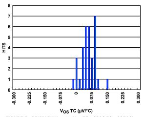
FIGURE 5. PRIMARY  $V_{SHUNT} V_{OS} TC (-40 \,^{\circ}C TO +125 \,^{\circ}C)$
