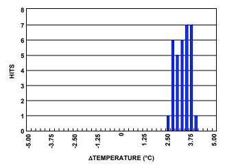
FIGURE 57. INTERNAL TEMPERATURE ACCURACY AT T = +25°C
