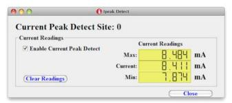
FIGURE 66. THE ISL28025 TRACKS MINIMUM AND MAXIMUM AVERAGE CURRENT READINGS
