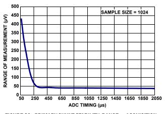
FIGURE 60. PRIMARY SHUNT STABILITY: RANGE vs ACQUISITION TIME
