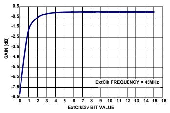
FIGURE 81. EXTERNAL CLOCK vs EXTERNAL BIT VALUE
