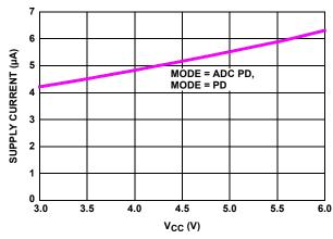
FIGURE 40. SUPPLY CURRENT vs SUPPLY VOLTAGE (POWER-DOWN MODES)
