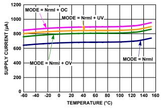
FIGURE 37. SUPPLY CURRENT vs TEMPERATURE
