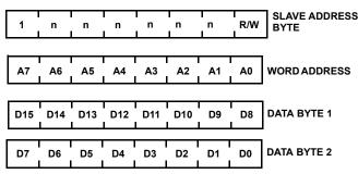
FIGURE 74. SLAVE ADDRESS, WORD ADDRESS AND DATA BYTES
