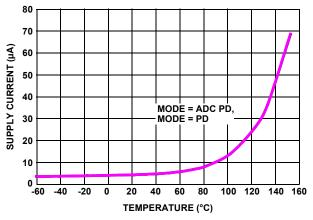
FIGURE 38. POWER-DOWN SUPPLY CURRENT vs TEMPERATURE
