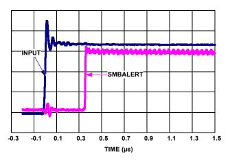
FIGURE 58. OV OR UV OR OC ALERT RESPONSE TIME
