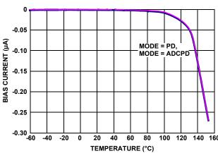
FIGURE 42. PRIMARY V<sub>SHUNT</sub> BIAS CURRENT vs TEMPERATURE (POWER-DOWN MODE)
