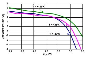
FIGURE 56. INTERNAL TEMPERATURE ACCURACY vs V<sub>CC</sub>
