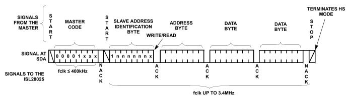
FIGURE 75. BYTE TRANSACTION SEQUENCE FOR INITIATING DATA RATES ABOVE 400kbps
