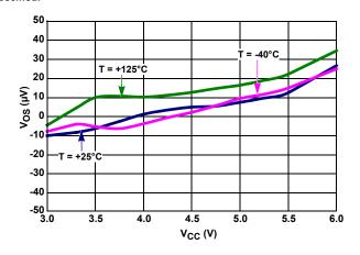
FIGURE 4. PRIMARY  $V_{SHUNT} V_{OS}$  vs VCC
