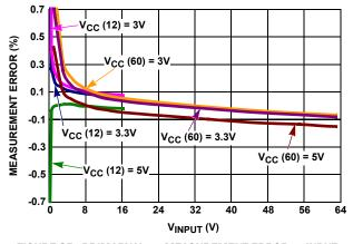
FIGURE 25. PRIMARY  $V_{\mbox{\scriptsize BUS}}$  MEASUREMENT ERROR vs INPUT
