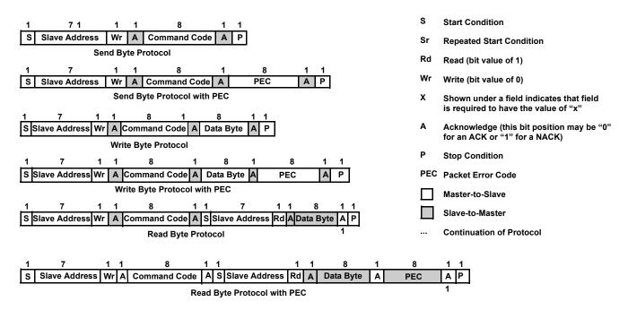
FIGURE 64. READ/WRITE SMBus PROTOCOLS WITH AND WITHOUT PEC
