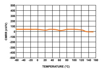
FIGURE 8. PRIMARY V<sub>SHUNT</sub> CMRR vs TEMPERATURE (CMV = 0V TO 60V)
