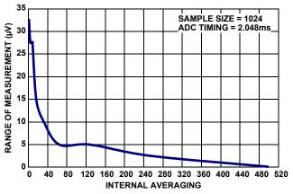
FIGURE 62. PRIMARY SHUNT STABILITY: RANGE vs INTERNAL **AVERAGING**
