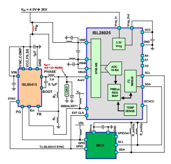
FIGURE 77. SIMPLIFIED SCHEMATIC OF THE ISL28025 SYNCHRONIZED TO A MCU SYSTEM CLOCK
