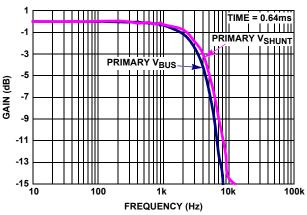
FIGURE 18. PRIMARY  $V_{SHUNT}$  and  $V_{BUS}$  vs frequency
