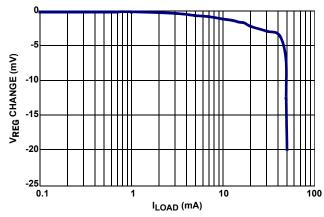
FIGURE 52. V<sub>REG</sub> OUTPUT vs CURRENT LOAD
