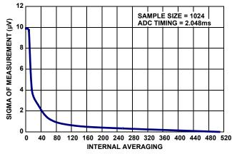
FIGURE 61. PRIMARY SHUNT STABILITY: STDEV vs INTERNAL **AVERAGING**
