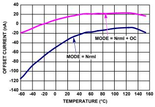
FIGURE 43. PRIMARY  $V_{SHUNT}$  BIAS CURRENT OFFSET vs **TEMPERATURE**
