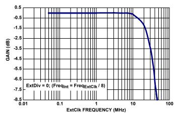
FIGURE 80. EXTERNAL CLOCK BANDWIDTH vs MEASUREMENT **ACCURACY**
