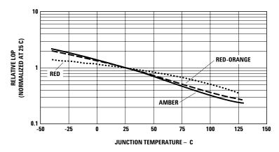
Figure 8. Relative light output vs. junction temperature
