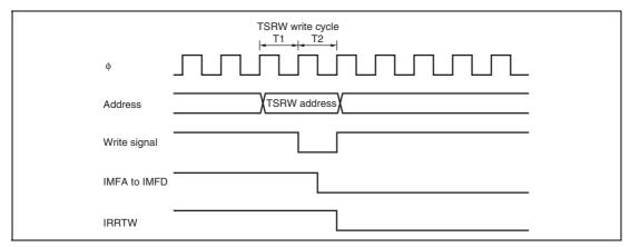
Figure 11.23 Timing of Status Flag Clearing by CPU
