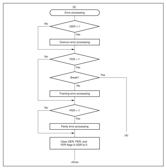
Figure 13.8 Sample Serial Reception Data Flowchart (Asynchronous Mode)(2)
