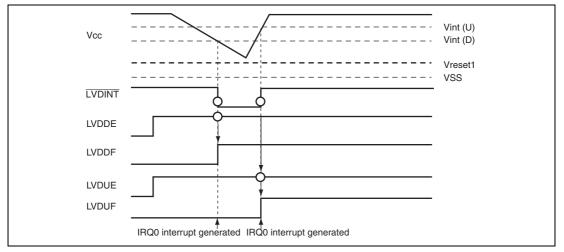
Figure 15.4 Operational Timing of LVDI Circuit
