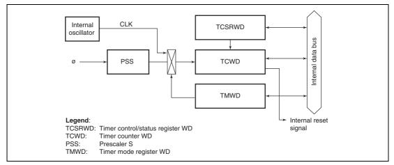
Figure 12.1 Block Diagram of Watchdog Timer
