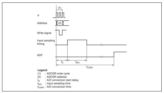
Figure 14.2 A/D Conversion Timing
