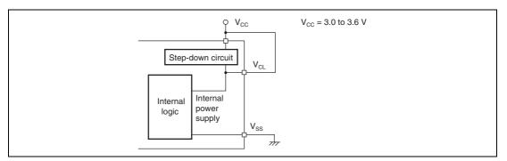
Figure 16.2 Power Supply Connection when Internal Step-Down Circuit is Not Used
