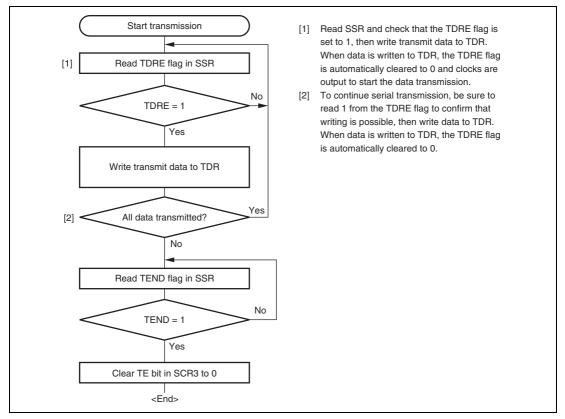
Figure 13.11 Sample Serial Transmission Flowchart (Clocked Synchronous Mode)
