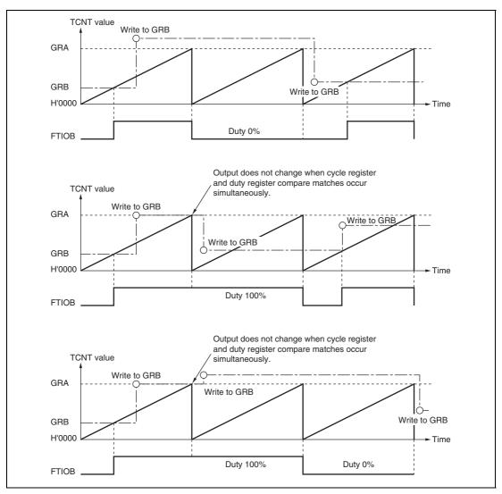
Figures 11.12 and 11.13 show examples of the output of PWM waveforms with duty cycles of 0% and 100%.
