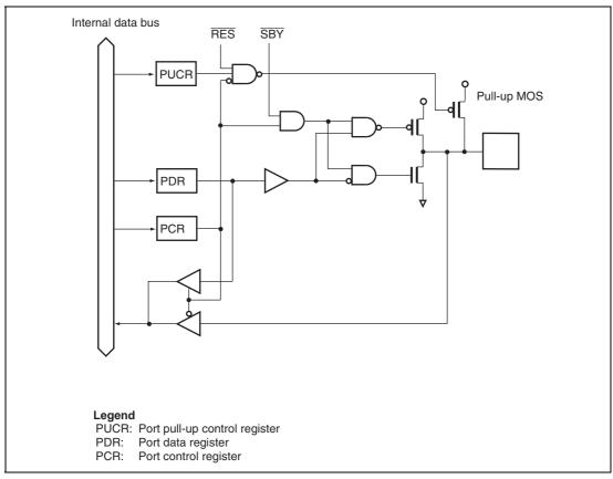
Figure B.5 Port 1 Block Diagram (P11)
