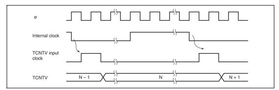
Figure 10.2 Increment Timing with Internal Clock
