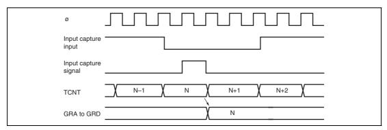
Figure 11.17 Input Capture Input Signal Timing
