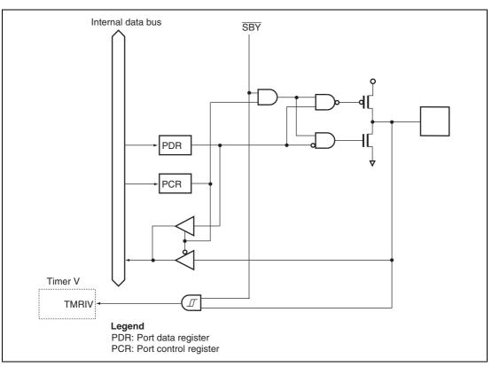
Figure B.16 Port 7 Block Diagram (P74)
