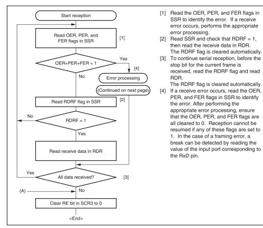
Figure 13.8 Sample Serial Reception Data Flowchart (Asynchronous Mode)(1)
