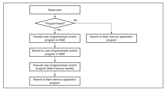
Figure 7.2 Programming/Erasing Flowchart Example in User Program Mode
