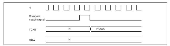
Figure 11.18 Timing of Counter Clearing by Compare Match
