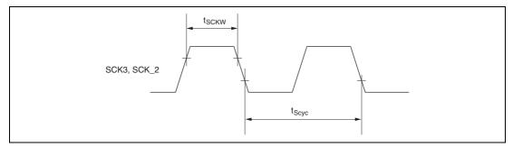
Figure 18.4 SCK3 Input Clock Timing
