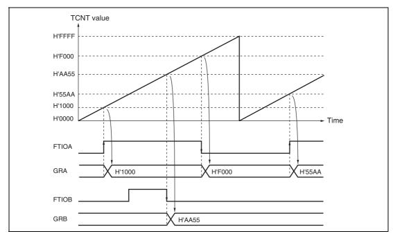
Figure 11.7 Input Capture Operating Example
