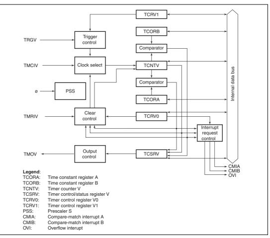
Figure 10.1 Block Diagram of Timer V
