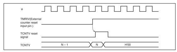
Figure 10.8 Clear Timing by TMRIV Input
