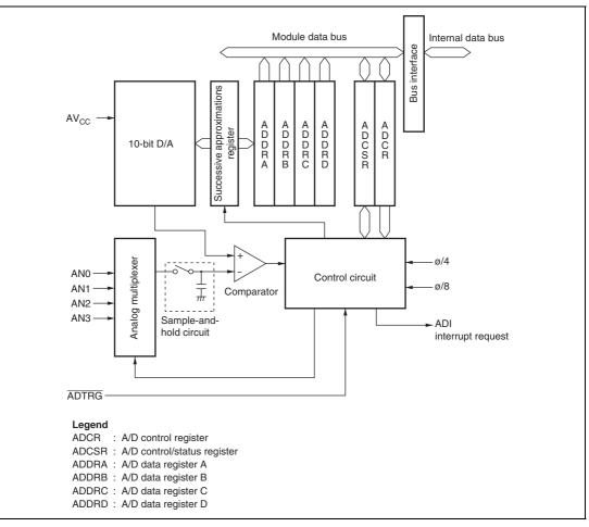
Figure 14.1 Block Diagram of A/D Converter
