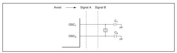
Figure 5.7 Example of Incorrect Board Design
