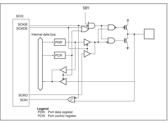
Figure B.8 Port 2 Block Diagram (P20)
