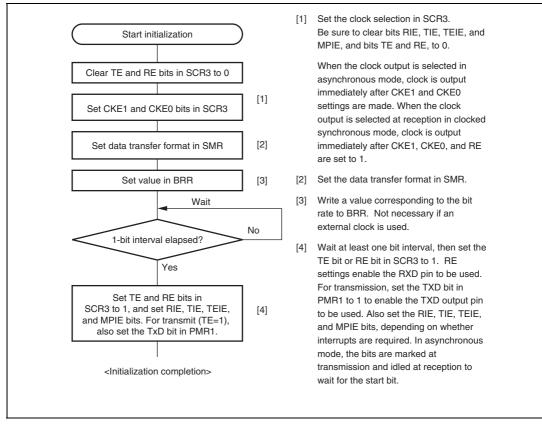
Figure 13.4 Sample SCI3 Initialization Flowchart
