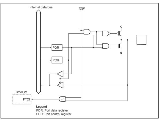
Figure B.22 Port 8 Block Diagram (P80)
