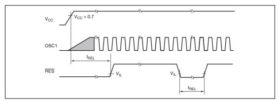
Figure 18.2 RES Low Width Timing
