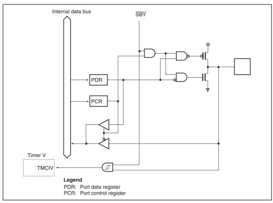
Figure B.15 Port 7 Block Diagram (P75)
