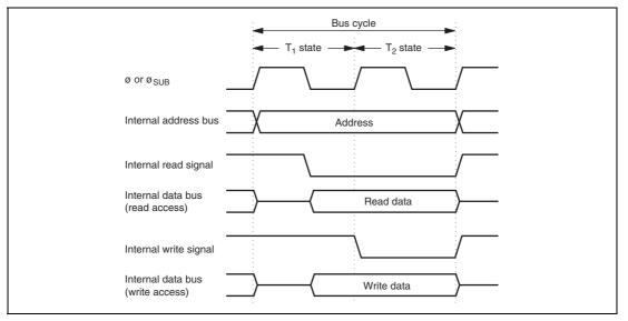
Figure 2.9 On-Chip Memory Access Cycle
