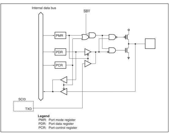
Figure B.6 Port 2 Block Diagram (P22)
