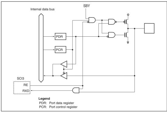
Figure B.7 Port 2 Block Diagram (P21)
