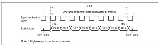
Figure 13.9 Data Format in Clocked Synchronous Communication
