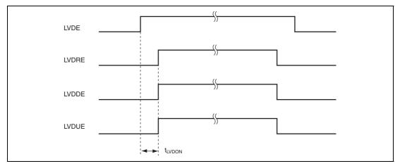
Figure 15.5 Timing for Operation/Release of Low-Voltage Detection Circuit
