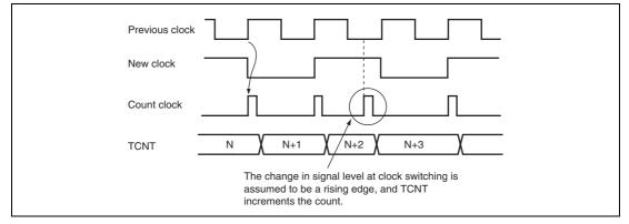
Figure 11.25 Internal Clock Switching and TCNT Operation
