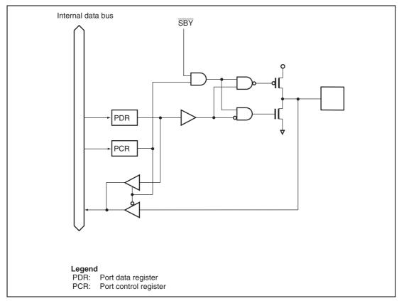
Figure B.17 Port 7 Block Diagram (P73)
