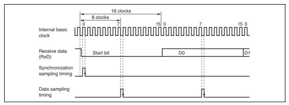
Figure 13.19 Receive Data Sampling Timing in Asynchronous Mode
