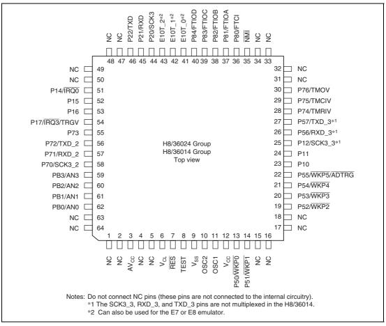
Figure 1.2 Pin Arrangement (FP-64E)
