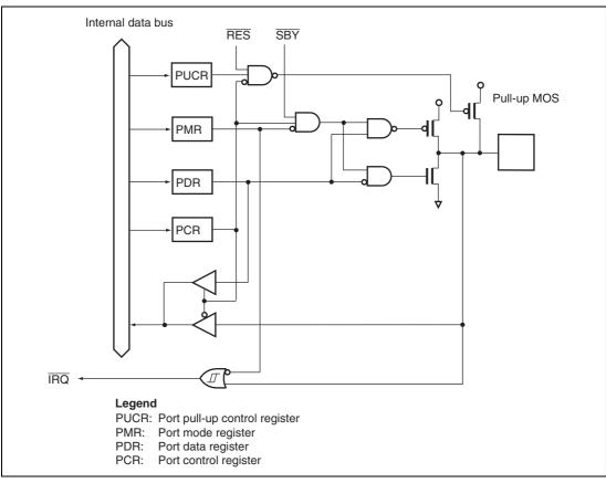
Figure B.2 Port 1 Block Diagram (P14)
