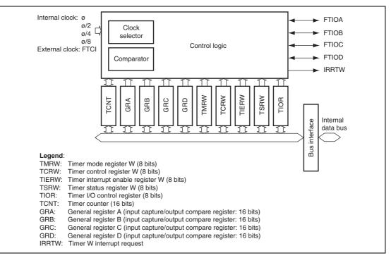
Figure 11.1 Timer W Block Diagram
