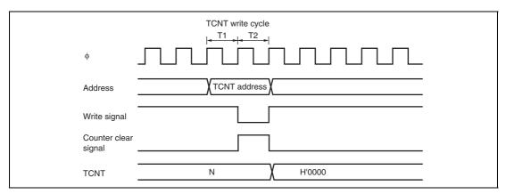
Figure 11.24 Contention between TCNT Write and Clear
