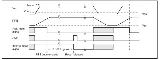
Figure 15.2 Operational Timing of Power-On Reset Circuit
