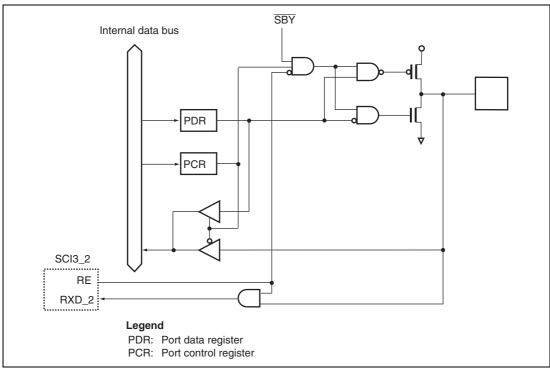
Figure B.19 Port 7 Block Diagram (P71)
