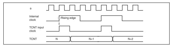
Figure 11.14 Count Timing for Internal Clock Source
