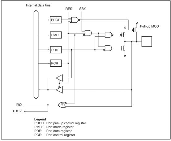
Figure B.1 Port 1 Block Diagram (P17)
