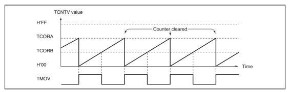
Figure 10.9 Pulse Output Example
