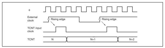
Figure 11.15 Count Timing for External Clock Source
