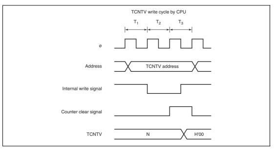
Figure 10.11 Contention between TCNTV Write and Clear
