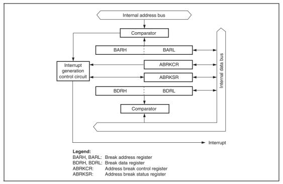
Figure 4.1 Block Diagram of Address Break
