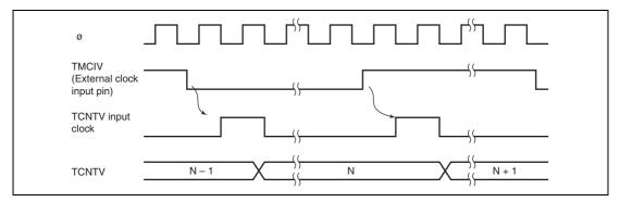
Figure 10.3 Increment Timing with External Clock
