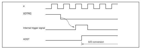
Figure 14.3 External Trigger Input Timing
