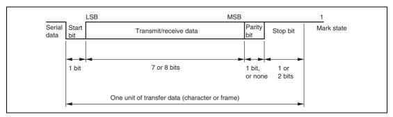
Figure 13.2 Data Format in Asynchronous Communication
