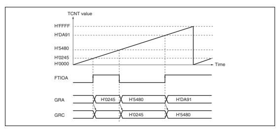
Figure 11.8 Buffer Operation Example (Input Capture)
