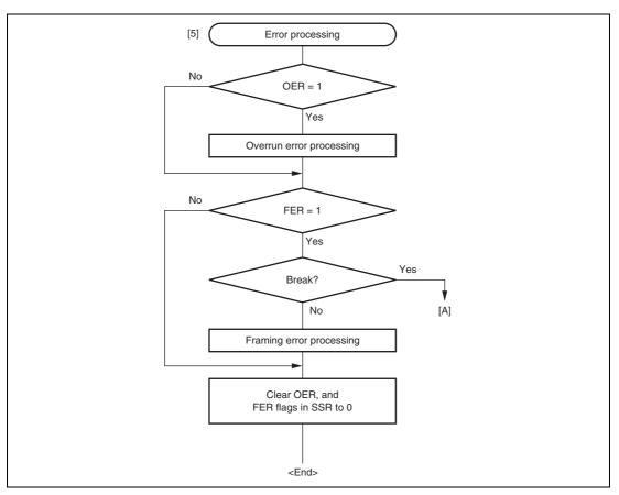
Figure 13.17 Sample Multiprocessor Serial Reception Flowchart (2)
