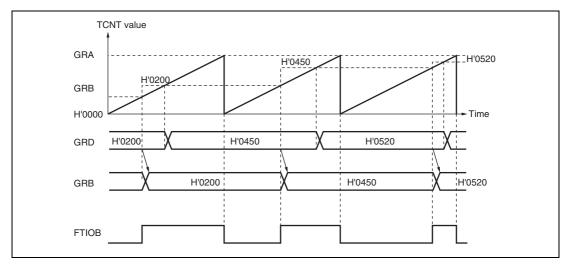
Figure 11.11 Buffer Operation Example (Output Compare)
