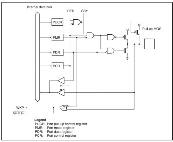
Figure B.12 Port 5 Block Diagram (P55)
