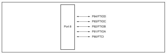
Figure 9.5 Port 8 Pin Configuration
