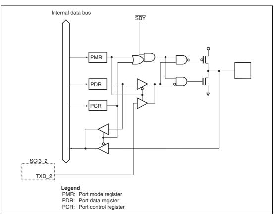
Figure B.18 Port 7 Block Diagram (P72)
