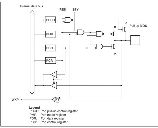
Figure B.13 Port 5 Block Diagram (P54 to P50)
