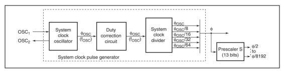
Figure 5.1 Block Diagram of Clock Pulse Generators
