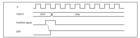
Figure 10.4 OVF Set Timing
