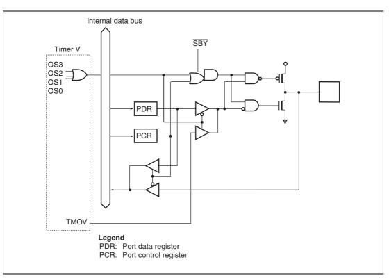
Figure B.14 Port 7 Block Diagram (P76)
