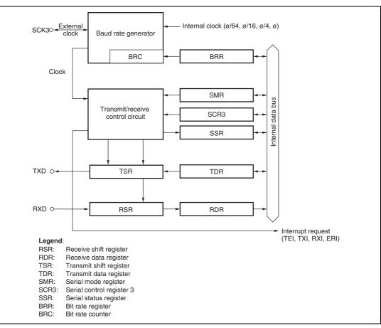
Figure 13.1 Block Diagram of SCI3
