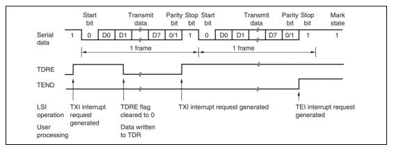
Figure 13.5 Example of SCI3 Transmission in Asynchronous Mode (8-Bit Data, Parity, One Stop Bit)
