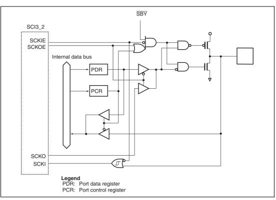
Figure B.20 Port 7 Block Diagram (P70)
