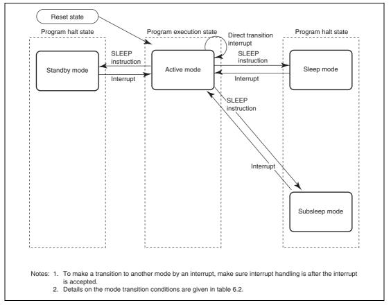
Figure 6.1 Mode Transition Diagram
