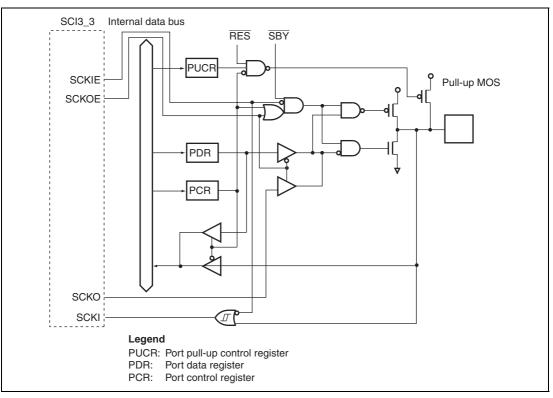
Figure B.4 Port 1 Block Diagram (P12) (H8/36024)
