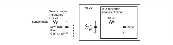
Figure 14.6 Analog Input Circuit Example
