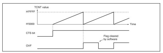
Figure 11.2 Free-Running Counter Operation
