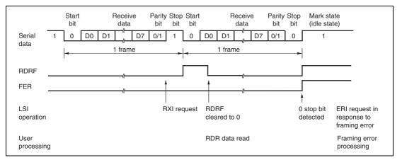
Figure 13.7 Example of SCI3 Reception in Asynchronous Mode (8-Bit Data, Parity, One Stop Bit)
