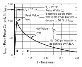
Fig. 3 - Pulse Waveform
