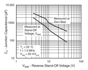
Fig. 4 - Typical Junction Capacitance
