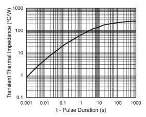
Fig. 5 - Typical Transient Thermal Impedance
