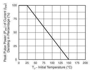
Fig. 2 - Pulse Derating Curve
