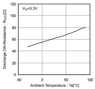
Figure 19. Discharge ON-Resistance vs Ambient Temperature
