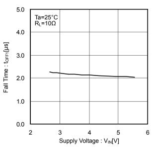
Figure 14. Output Fall Time vs Supply Voltage
