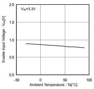
Figure 6. EN Input Voltage vs Ambient Temperature
