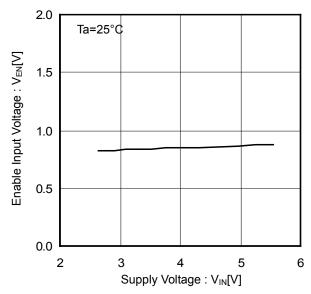
Figure 5. EN Input Voltage vs Supply Voltage
