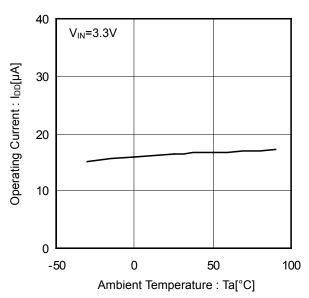
Figure 2. Operating Current vs Ambient Temperature (EN Enable)
