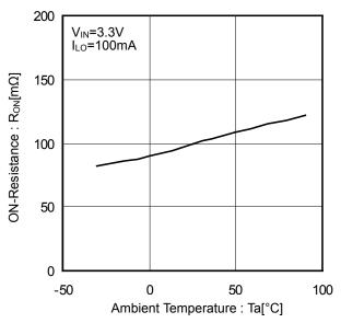
Figure 8. ON-Resistance vs Ambient Temperature
