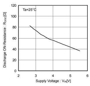
Figure 18. Discharge ON-Resistance vs Supply Voltage
