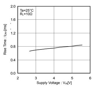
Figure 10. Output Rise Time vs Supply Voltage
