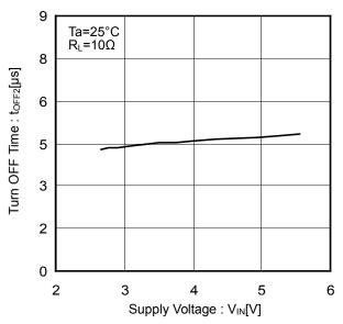
Figure 16. Output Turn OFF Time vs Supply Voltage
