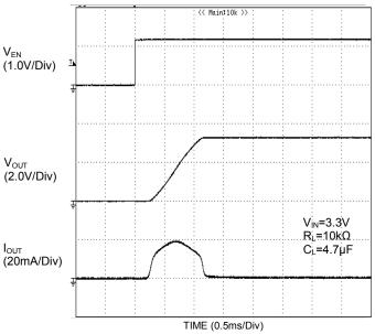
Figure 20. Output Turn ON Response (V<sub>IN</sub>=3.3V R<sub>L</sub>=10kΩ C<sub>L</sub>=4.7μF)
