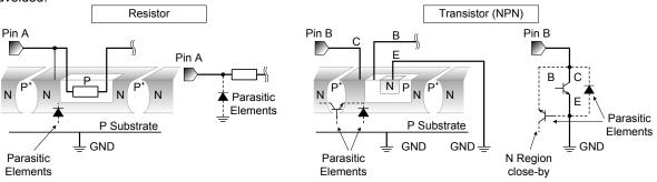
Figure 25. Example of monolithic IC structure
