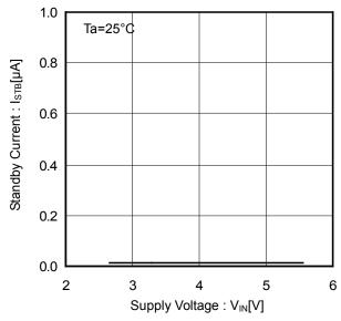
Figure 3. Standby Current vs Supply Voltage (EN Disable)
