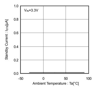
Figure 4. Standby Current vs Ambient Temperature (EN Disable)
