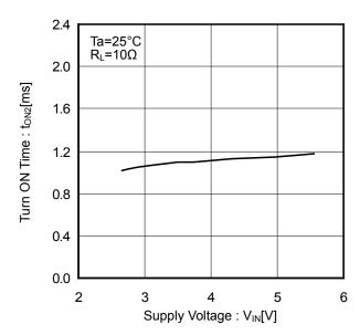
Figure 12. Output Turn ON Time vs Supply Voltage
