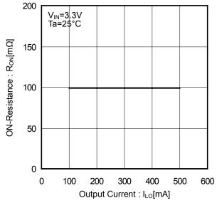
Figure 9. ON-Resistance vs Output Current
