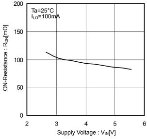
Figure 7. ON-Resistance vs Supply Voltage
