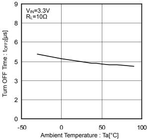
Figure 17. Output Turn OFF Time vs Ambient Temperature
