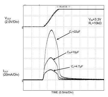
Figure 22. Rush Current Response  $(V_{IN}=3.3V R_L=10k\Omega)$
