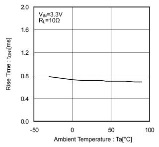
Figure 11. Output Rise Time vs Ambient Temperature
