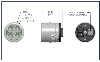
Diameter x H 35.0mm x 37.5mm (1.38" x 1.48") Maximum Cable Dia - 1.5mm<sup>2</sup> / 16 AWG
