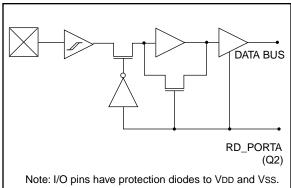
FIGURE 9-2: RA2 AND RA3 BLOCK DIAGRAM
