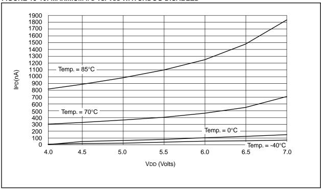
FIGURE 18-11: TYPICAL IPD vs. VDD WATCHDOG ENABLED 25°C
