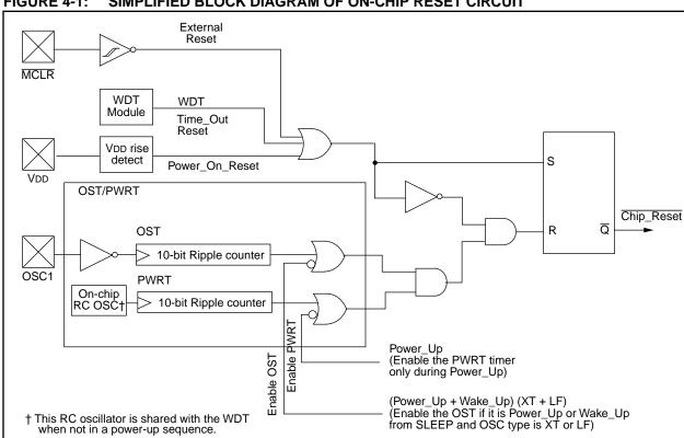
SIMPLIFIED BLOCK DIAGRAM OF ON-CHIP RESET CIRCUIT FIGURE 4-1:
