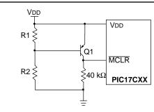
This brown-out circuit is less expensive, albeit less accurate. Transistor Q1 turns off when VDD is below a certain level such that:
