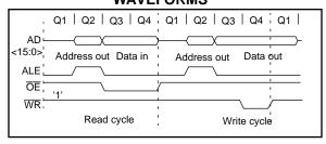
The system bus requires that there is no bus conflict (minimal leakage), so the output value (address) will be capacitively held at the desired value.
