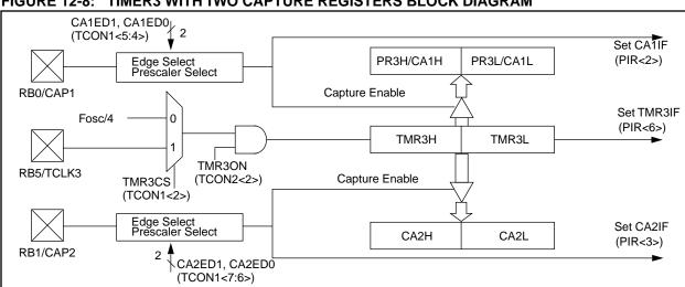
FIGURE 12-8: TIMER3 WITH TWO CAPTURE REGISTERS BLOCK DIAGRAM
