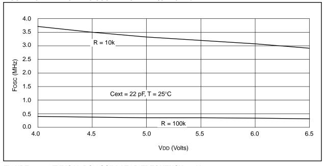
FIGURE 20-3: TYPICAL RC OSCILLATOR FREQUENCY vs. VDD
