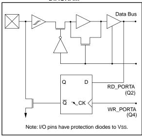
FIGURE 9-3: RA4 AND RA5 BLOCK DIAGRAM
