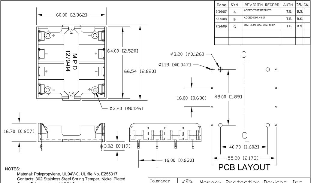
Cover: Polypropylene, UL94V-0 Heat Deflection Temperature: 90°C
