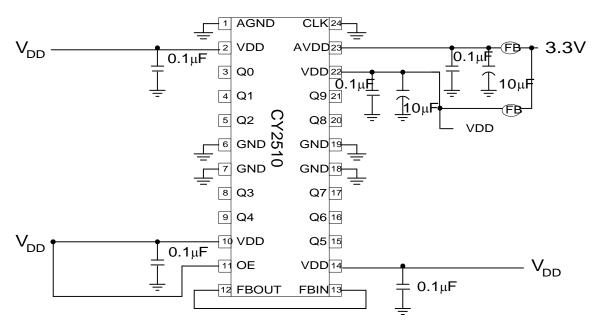
Figure 1. CY2510 Example Schematic
