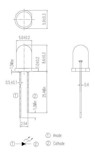
Note: Tolerances unless dimensions ±0.25mm
