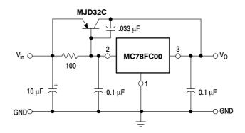
Figure 7. Current Boost Circuit
