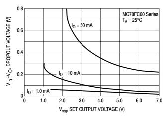
Figure 2. Dropout versus Set Output Voltage
