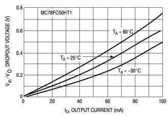
Figure 4. Dropout Voltage versus Output Current
