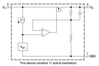
Figure 1. Representative Block Diagram
