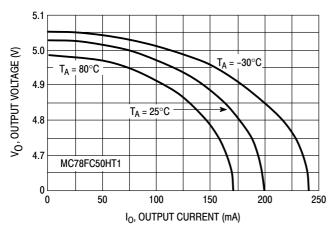
Figure 1. Output Voltage versus Output Current
