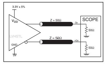
**Output Load AC Test Circuit**
