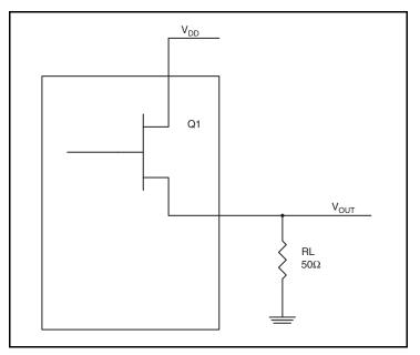
Figure 4. LVHSTL Driver Circuit and Termination
