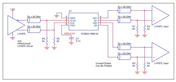
Figure 3. 85211BI-03 LVHSTL Buffer Schematic Example
