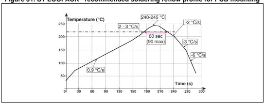
Note: Minimize air convection currents in the reflow oven to avoid component movement.
