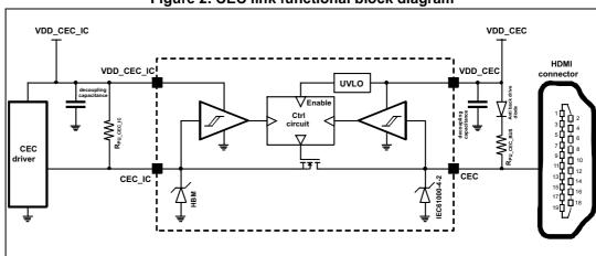
Figure 2. CEC link functional block diagram
