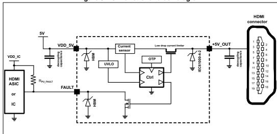
Figure 9. +5V functional block diagram
