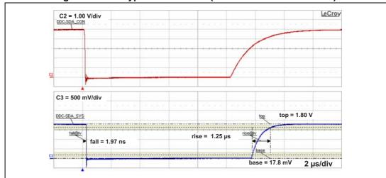
Figure 16. DDC typical waveforms (cable to IC communication)
