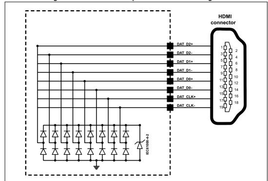
Figure 10. TMDS lines ESD protection functional diagram
