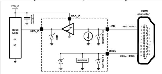
Figure 7. HEAC / HPD / Utility functional block diagram
