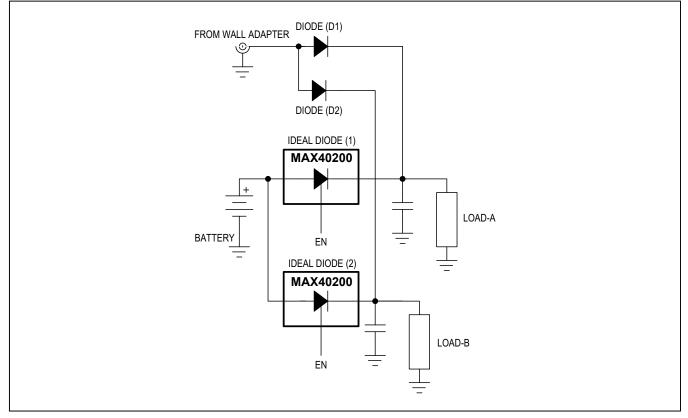
Figure 2. Diode ORing Circuit 2
