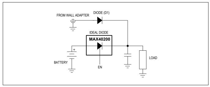
Figure 1. Diode ORing Circuit 1
