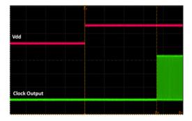
Figure 17. Startup Waveform vs. Vdd
