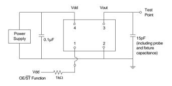
**Figure 2. Test Circuit**
