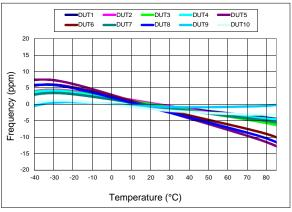
Figure 9. Frequency vs Temperature
