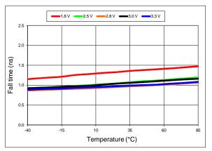
Figure 13. 20%-80% Fall Time vs Temperature
