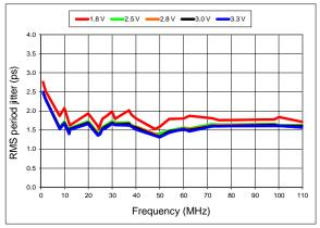
Figure 10. RMS Period Jitter vs Frequency
