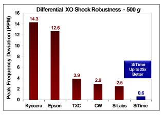
Figure 6. Shock Robustness<sup>[6]</sup>
