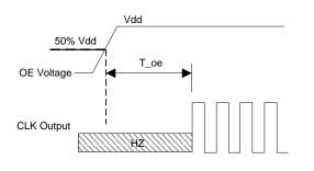
T\_oe: Time to re-enable the clock output
