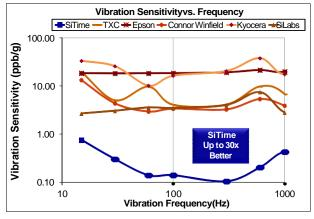
Figure 5. Vibration Robustness<sup>[5]</sup>
