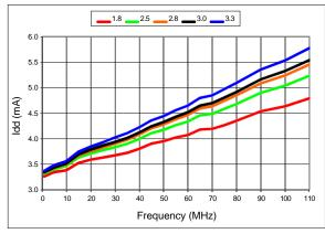
Figure 8. Idd vs Frequency
