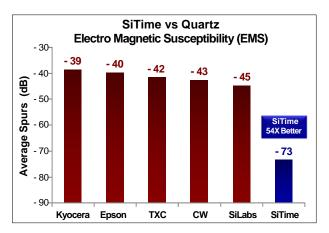
Figure 3. Electro Magnetic Susceptibility (EMS)<sup>[3]</sup>
