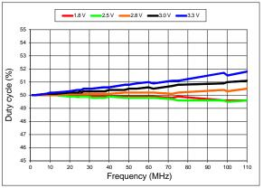
Figure 11. Duty Cycle vs Frequency
