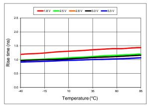
Figure 12. 20%-80% Rise Time vs Temperature
