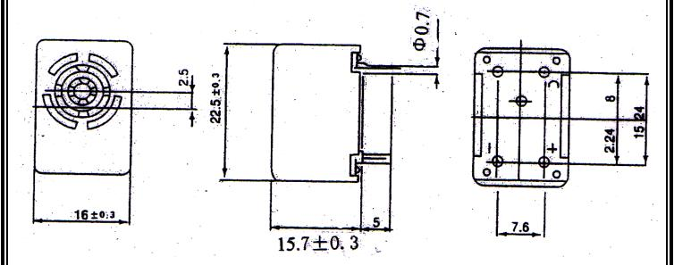
Must connect "-" to ground; "+" & "C" to positive voltage for operation.
