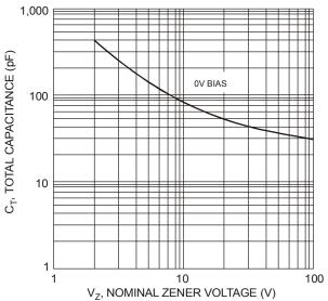
Fig. 2 Typical Total Capacitance vs. Nominal Zener Voltage
