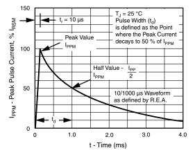
Fig. 3 - Pulse Waveform
