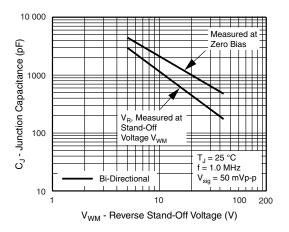
Fig. 4 - Typical Junction Capacitance
