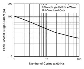
Fig. 6 - Maximum Non-Repetitive Forward Surge Current
