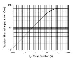
Fig. 5 - Typical Transient Thermal Impedance
