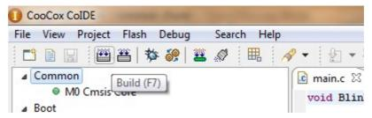
After building the project initiate debug to download the program to the target. Press F5 to resume the program execution. This blinks the D2 on mX-LPC11U14-S board.
