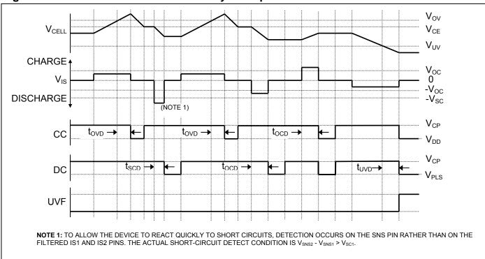
Figure 18. Lithium-Ion Protection Circuitry Example Waveforms
