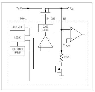
Figure 19. Closed-Loop Tracking
