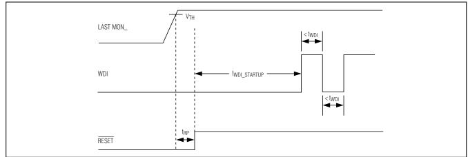
Figure 6. Normal Watchdog Startup Sequence
