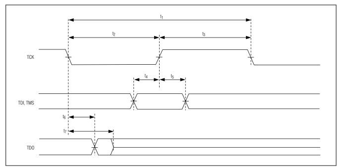
Figure 2. JTAG Timing Diagram
