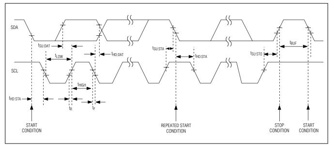
Figure 1. I<sup>2</sup>C/SMBus Timing Diagram
