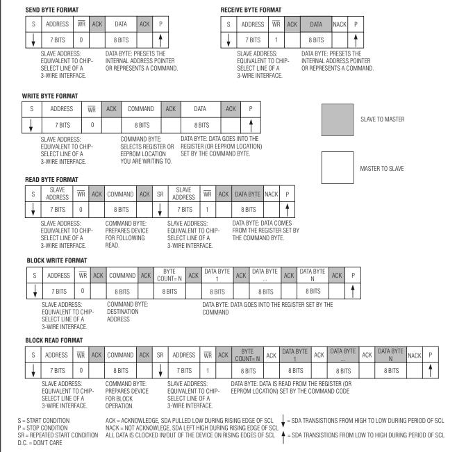
Figure 12. I<sup>2</sup>C/SMBus Protocols
