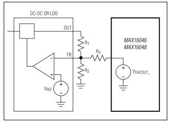
Figure 15. Connections for Margining Using Feedback Method
