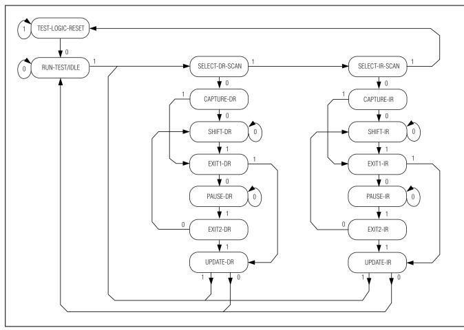
Figure 14. TAP Controller State Diagram
