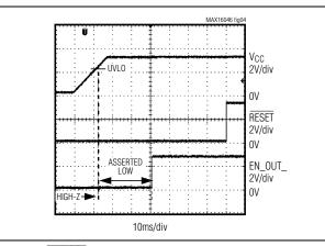
Figure 4. RESET and EN\_OUT\_ During Power-Up, EN\_OUT\_ Is in Push-Pull Active-High Configuration
