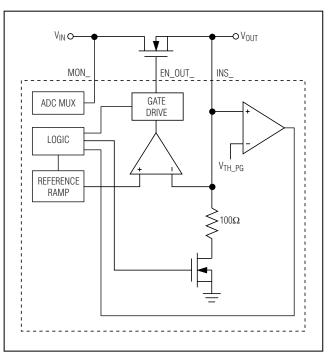
Figure 5. Closed-Loop Tracking
