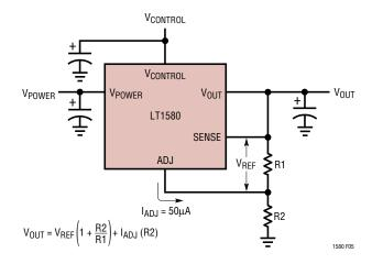
Figure 5. Setting Output Voltage
