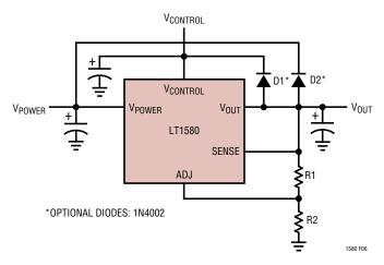
Figure 6. Optional Clamp Diodes Protect Against Input Crowbar Circuits
