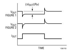
Figure 3. Remote Sensing Improves Load Regulation
