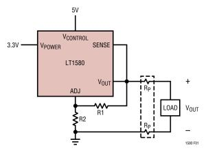
Figure 1. Conventional Load Sensing
