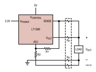
Figure 2. Remote Load Sensing
