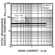
Fig.2 Static Drain-Source On-State Resistance vs. Drain Current
