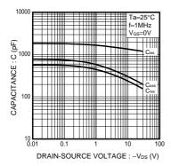
Fig.7 Typical Capacitance vs. Drain-Source Voltage
