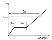
Fig.13 Gate Charge Waveform
