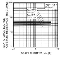
Fig.4 Static Drain-Source On-State vs. Drain Current
