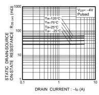
Fig.5 Static Drain-Source On-State vs. Drain Current
