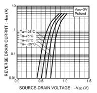
Fig.6 Reverse Drain Current Source-Drain Current
