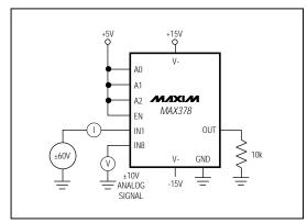
Figure 4. Input Leakage Current (Overvoltage)
