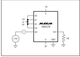
Figure 5. Input Leakage Current (with Power Supplies OFF)
