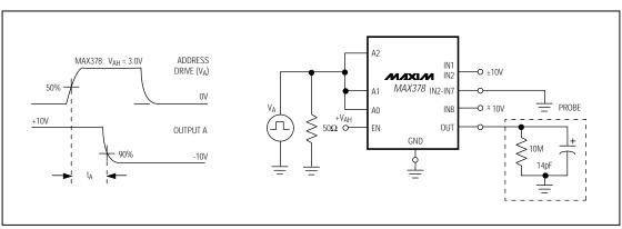
Figure 1. Access Time vs. Logic Level (High)
