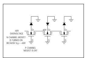
Figure 7. -60V Overvoltage with Multiplexer Power OFF
