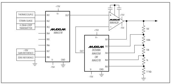
Figure 6. Typical Data Acquisition Front End
