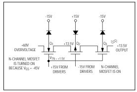
Figure 10. +60V Overvoltage Input to the ON Channel
