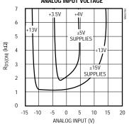
NOTE: Typical R<sub>DS(ON)</sub> match @ +10V Analog in (±15V supplies) = 2% for lowest to highest R<sub>DS(ON)</sub> channel; @ -10V Analog in, match = 3%.
