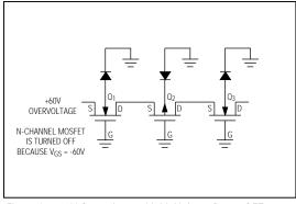
Figure 8. +60V Overvoltage with Multiplexer Power OFF
