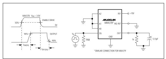
Figure 3. Enable Delay (ton(EN), toff(EN))
