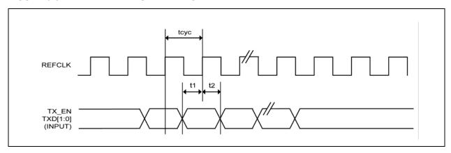
FIGURE 6-7: RMII RECEIVE TIMING
