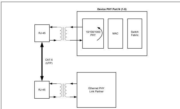
The following programming steps and register settings are for remote PHY loopback mode for 1000BASE-T Master Mode, 1000BASE-T Slave Mode, 100BASE-TX Mode, and 10BASE-T Mode.
