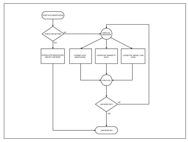
For 1000BASE-T mode, auto-negotiation is always required to establish a link. During 1000BASE-T auto-negotiation, the master and slave configuration is first resolved between link partners. Then the link is established with the highest common capabilities between link partners.
