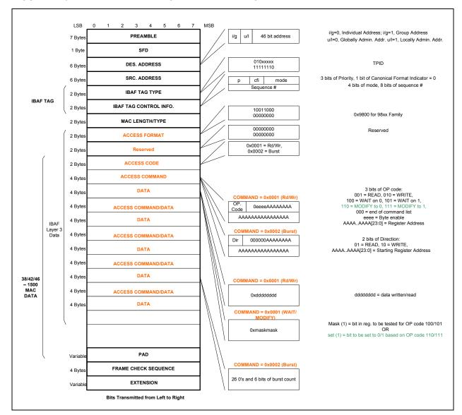
FIGURE 4-16: IN-BAND MANAGEMENT FRAME FORMAT
