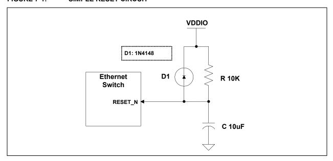
Figure 7-2 illustrates a reset circuit recommended for applications where reset is driven by another device, such as a CPU. At power-on reset, R, C and D1 provide the necessary ramp rise time to reset the KSZ9477S. The RST\_OUT\_N from the CPU provides a warm reset after power-up.
