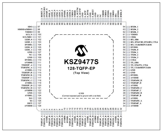
**Note:** When an "\_N" is used at the end of the signal name, it indicates that the signal is active low. For example, **RESET\_N** indicates that the reset signal is active low.
