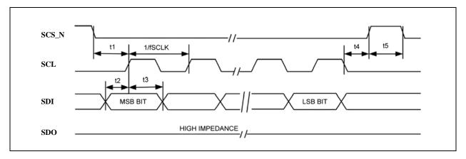
FIGURE 6-10: SPI DATA OUTPUT TIMING
