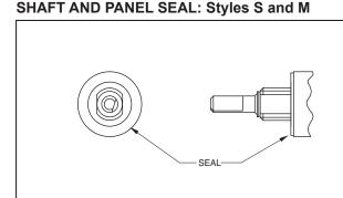
Shaft and panel seal switches are watertight to the panel. They are not totally process sealed like the Style "T". Panel is sealed by a gasket at the base of the bushing. Shaft is sealed by an O-ring inside the bushing. After mounting, seals do not alter switch dimensions. See Style "S" (standard switches) and Style "M" (military switches) in the Choices and Limitations chart.
