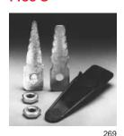
communications cable and a conductor such as a strap, bar, or wire. The connector consists of five parts: lower member (base), upper member (top), two securing nuts (lock nuts) and a plastic shoe to aid connector insertion and to protect conductors. The base teeth are set
