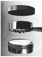
Protecting a buried service wire splice is now easier than ever with the SLiC Buried Service Wire Kit. The BSW kit is a three-part, rigid body closure that self-encapsulates two- and fivepair buried service wire. It has a builtin bonding system that bonds the buried service wire shield as the splice is put together—and it contains a revolutionary new sealant.
