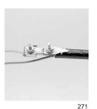
fiberglass strength members. The connector is a version of the 4460-D Connector Assembly which utilizes two additional plates to capture and secure the strength members. Its current-carrying capacity is equal to or better than aluminum-shielded fiber optic cable and can be used on all cables with 20.3 mm (0.8") or smaller O.D. RUS Listed.
