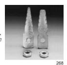
communications cable and a conductor such as a strap, bar, or wire. The connector consists of four parts: lower member (base), upper member (top), and two securing nuts (lock nuts). The base teeth are set at such an angle as to permit easy insertion under the cable shield. Top and base members are made of tin-plated tempered brass, slightly curved to exert a continuous spring force on sheath and shield after clamping.
