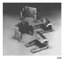
Designed to reduce closure support costs. The rack clips permit fast, multi-positioning of industry standard manhole racks or uni-struts and hooks to facilitate support of a closure. Two supports per set.
