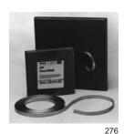
firmly, 25T Braid provides low electrical resistance connections for dependable shield bonding, and its physical strength contributes to strain relief across spliced cables, 25T Braid is 13 mm (1/2") wide, and is supplied in 7.6 m (25') rolls.
