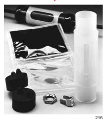
The Scotchcast Buried Service Wire Splice Kit 3832 will accommodate inline and butt splices of up to fivepair filled or unfilled service wire. One "A" size bag of 4403 encapsulant and a split bolt are provided with the kit. Once the compound has been poured, an outer tube is rotated over the barrel opening to seal the unit, requiring no waiting for the compound to cure before the kit is buried.
