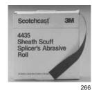
sheath greatly enhances the bond between the compound and sheath. Since the strip is 25.4 mm (1") wide, it encourages the craftsperson to scuff around the sheath rather than along it, thus eliminating moisture paths along the sheath, and also makes it easy to get into tight places.
