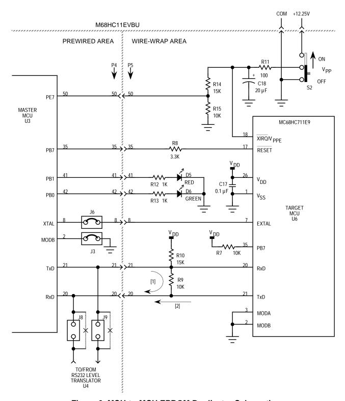
Figure 6. MCU-to-MCU EPROM Duplicator Schematic
