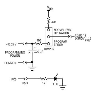
Figure 8. PC-to-MCU Programming Circuit
