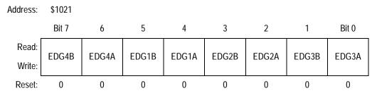
Figure 9-3. Timer Control Register 2 (TCTL2)
