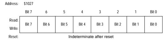
Figure 9-26. Pulse Accumulator Count Register (PACNT)
