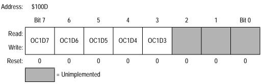
Figure 9-14. Output Compare 1 Data Register (OC1D)
