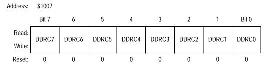
Figure 6-6. Port C Data Direction Register (DDRC)
