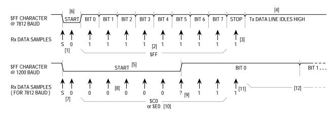
Figure 2. Automatic Detection of Baud Rate
