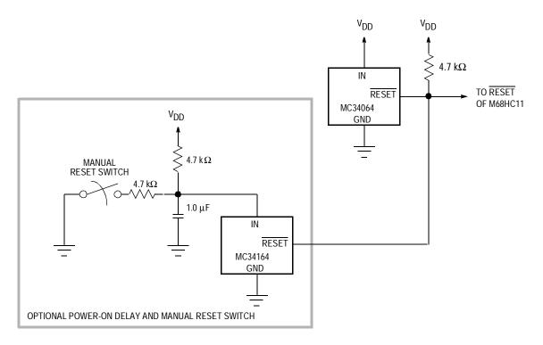
Figure 2-7. External Reset Circuit with Delay
