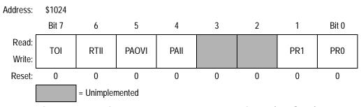
Figure 9-19. Timer Interrupt Mask 2 Register (TMSK2)
