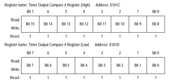
Figure 9-11. Timer Output Compare 4 Register Pair (TOC4)
