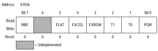
Figure 4-15. MC68HC711E20 EPROM Programming Control Register (EPROG)
