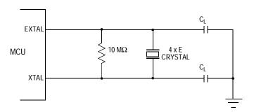
Figure 2-8. Common Parallel Resonant Crystal Connections
