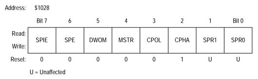
Figure 8-3. Serial Peripheral Control Register (SPCR)
