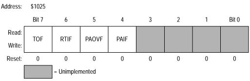
Figure 9-22. Timer Interrupt Flag 2 Register (TFLG2)
