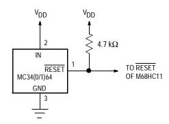
Figure 2-6. External Reset Circuit
