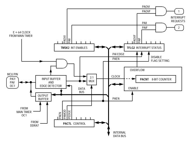
Figure 9-24. Pulse Accumulator
