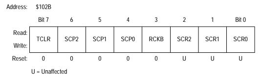
Figure 7-7. Baud Rate Register (BAUD)
