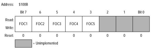
Figure 9-12. Timer Compare Force Register (CFORC)
