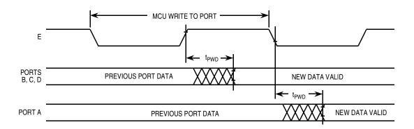
Figure 11-8. Port Write Timing Diagram
