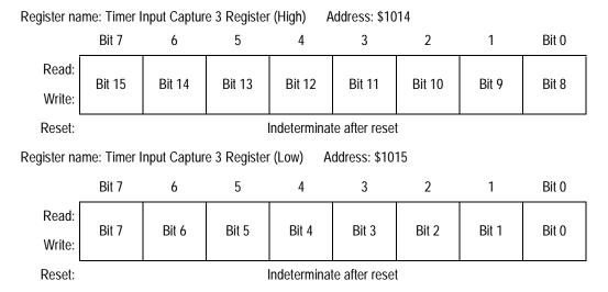
Figure 9-6. Timer Input Capture 3 Register Pair (TIC3)
