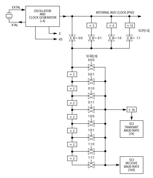
Figure 7-8. SCI Baud Rate Generator Block Diagram
