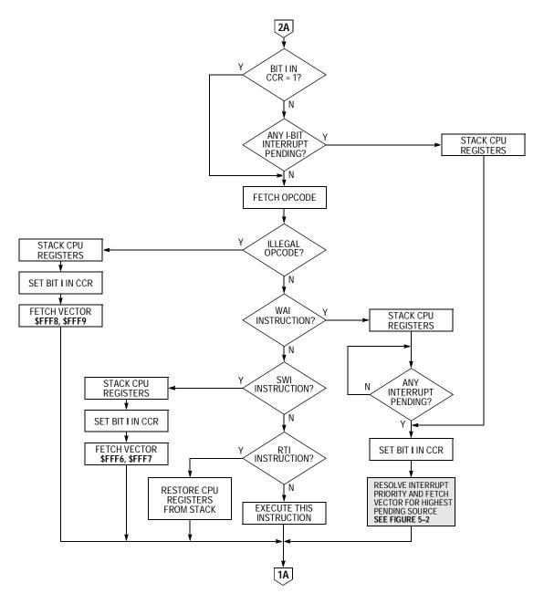
Figure 5-5. Processing Flow Out of Reset (Sheet 2 of 2)
