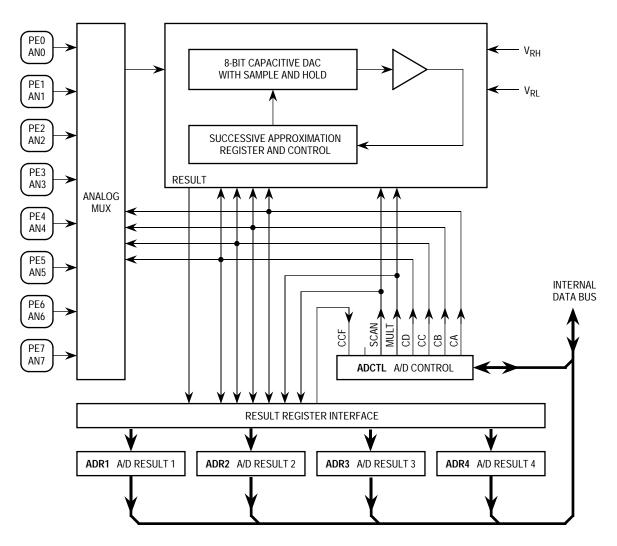
Figure 10-1. A/D Converter Block Diagram
