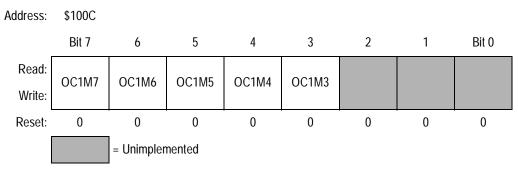
Figure 9-13. Output Compare 1 Mask Register (OC1M)
