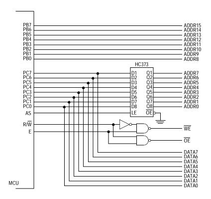
Figure 4-1. Address/Data Demultiplexing
