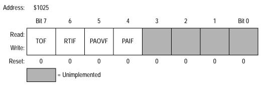
Figure 9-28. Timer Interrupt Flag 2 Register (TFLG2)
