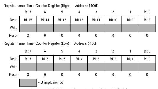
Figure 9-15. Timer Counter Register (TCNT)
