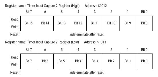
Figure 9-5. Timer Input Capture 2 Register Pair (TIC2)
