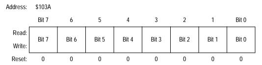
Figure 5-1. Arm/Reset COP Timer Circuitry Register (COPRST)
