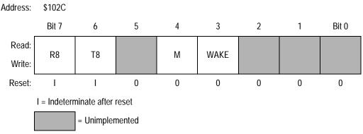
Figure 7-4. Serial Communications Control Register 1 (SCCR1)
