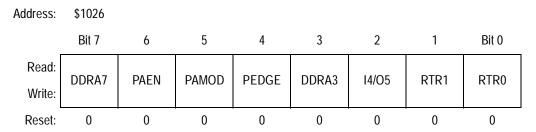
Figure 9-25. Pulse Accumulator Control Register (PACTL)
