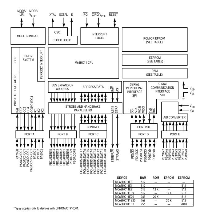
Figure 1-1. M68HC11 E-Series Block Diagram
