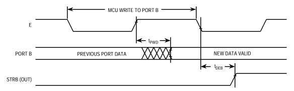
Figure 11-10. Simple Output Strobe Timing Diagram
