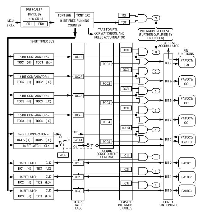
Figure 9-2. Capture/Compare Block Diagram
