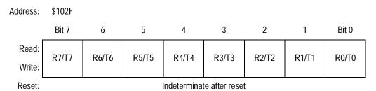
Figure 7-3. Serial Communications Data Register (SCDR)
