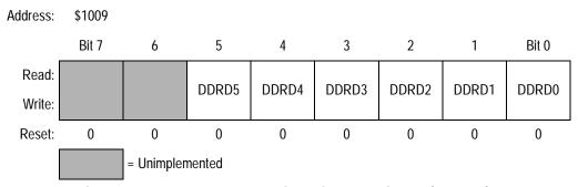
Figure 6-8. Port D Data Direction Register (DDRD)
