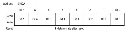
Figure 8-5. Serial Peripheral Data I/O Register (SPDR)
