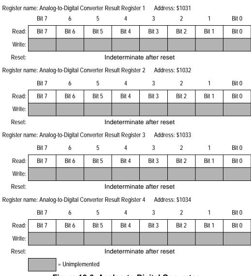
Figure 10-6. Analog-to-Digital Converter Result Registers (ADR1-ADR4)
