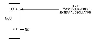
Figure 2-9. External Oscillator Connections
