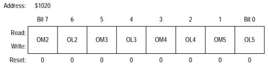
Figure 9-16. Timer Control Register 1 (TCTL1)
