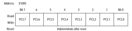
Figure 6-5. Port C Latched Register (PORTCL)
