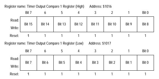
Figure 9-8. Timer Output Compare 1 Register Pair (TOC1)
