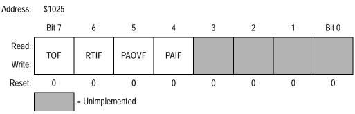
Figure 9-20. Timer Interrupt Flag 2 Register (TFLG2)
