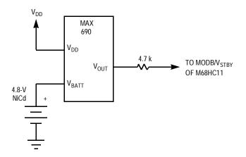
Figure 4-8. RAM Standby MODB/V<sub>STBY</sub> Connections
