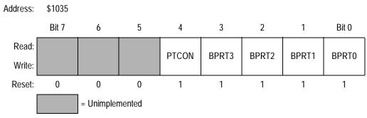
Figure 4-16. Block Protect Register (BPROT)
