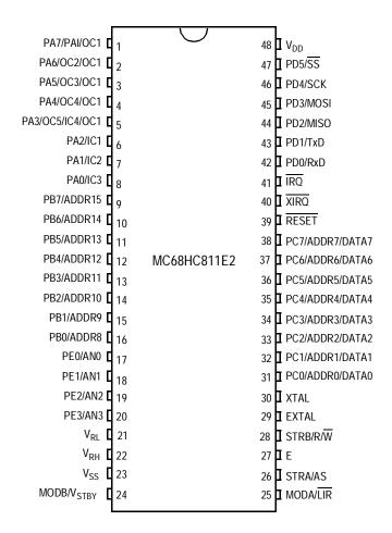
Figure 2-5. Pin Assignments for 48-Pin DIP (MC68HC811E2)
