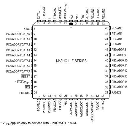
Figure 2-1. Pin Assignments for 52-Pin PLCC and CLCC
