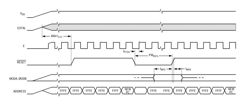
Figure 11-3. POR External Reset Timing Diagram
