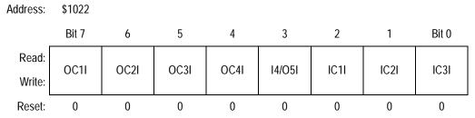
Figure 9-17. Timer Interrupt Mask 1 Register (TMSK1)
