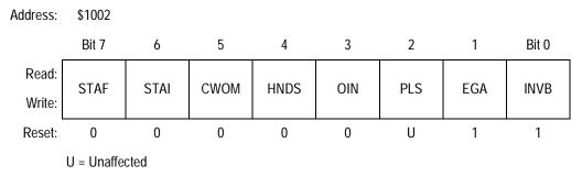
Figure 6-10. Parallel I/O Control Register (PIOC)
