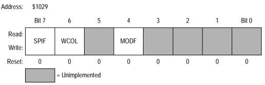
Figure 8-4. Serial Peripheral Status Register (SPSR)
