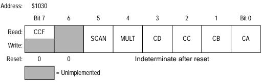
Figure 10-5. A/D Control/Status Register (ADCTL)
