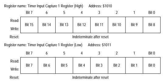
Figure 9-4. Timer Input Capture 1 Register Pair (TIC1)
