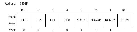
Figure 5-3. Configuration Control Register (CONFIG)
