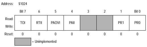
Figure 9-27. Timer Interrupt Mask 2 Register (TMSK2)
