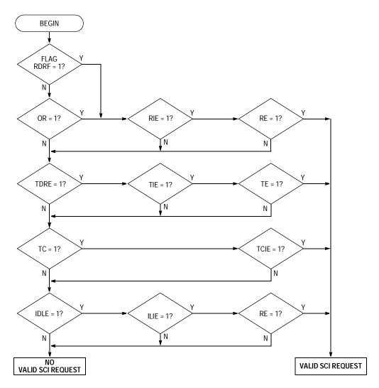
Figure 7-10. Interrupt Source Resolution Within SCI
