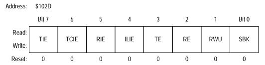
Figure 7-5. Serial Communications Control Register 2 (SCCR2)
