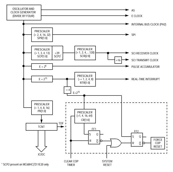
Figure 9-1. Timer Clock Divider Chains
