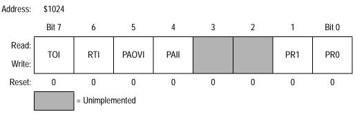
Figure 9-21. Timer Interrupt Mask 2 Register (TMSK2)
