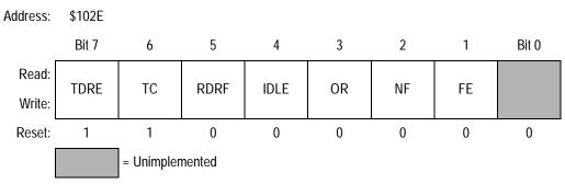
Figure 7-6. Serial Communications Status Register (SCSR)
