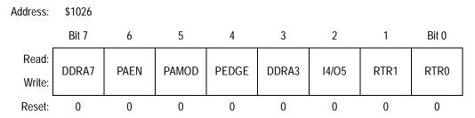
Figure 9-23. Pulse Accumulator Control Register (PACTL)
