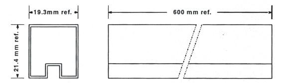
G8QN: 47 relays per tube, 36 tubes per box (1692 relays per box).
