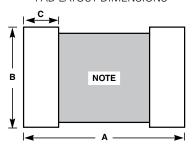
NOTE: Avoid metal runs in this area, parts not recommended for use in applications using Silver (Ag) epoxy paste.
