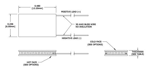
Ceramic Material Aluminum Nitride Ceramics Solder Construction: 232°C SnSb
