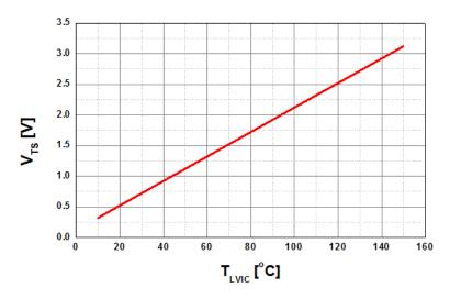
Figure 7. Temperature Profile of V<sub>TS</sub> (Typical)
