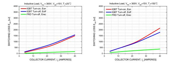
Figure 6. Switching Loss Characteristics
