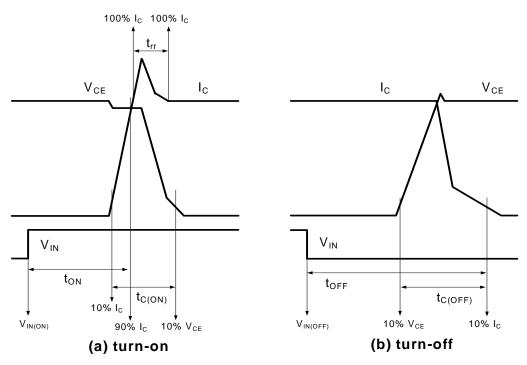
Figure 4. Switching Time Definition
