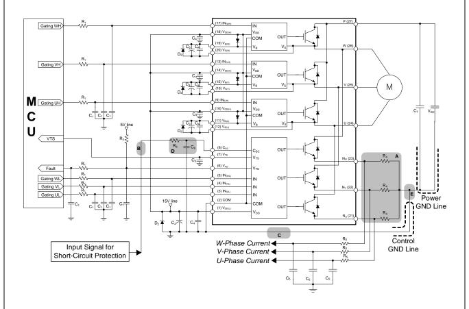
Figure 15. Typical Application Circuit
