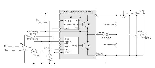
Figure 5. Example Circuit for Switching Test
