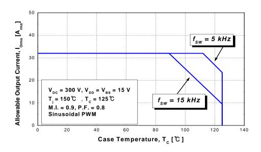
**Figure 8. Allowable Maximum Output Current**
