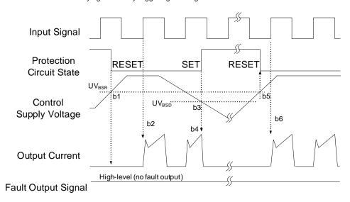
Figure 12. Under-Voltage Protection (High-Side)
