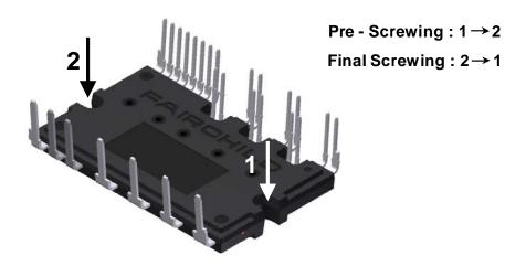
Figure 10. Mounting Screws Torque Order
