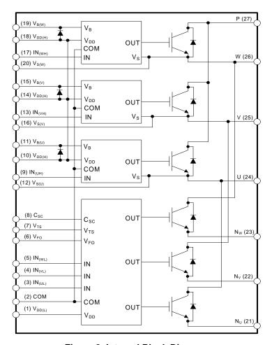
Figure 3. Internal Block Diagram
