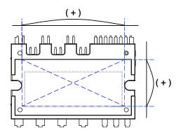
Figure 9. Flatness Measurement Position
