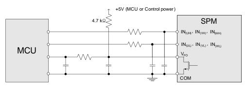
Figure 14. Recommended CPU I/O Interface Circuit
