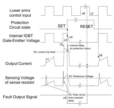
Figure 13. Short-Circuit Current Protection (Low-Side Operation only)
