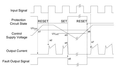
Figure 11. Under-Voltage Protection (Low-Side)
