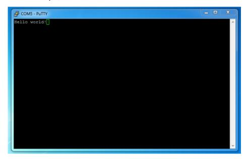
If you don't see anything, make sure you've connected the D0 pin to the D1 pin on the FT232H board.
