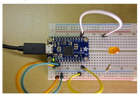
With this configuration pin **C0** will be a digital output that controls if the LED is on or off, depending on the level of the **C0** output. Pin **D7** will be a digital input that reads if it's at a high level (3-5 volts) or low level (ground).
