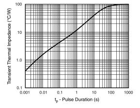
Fig. 5 - Typical Transient Thermal Impedance
