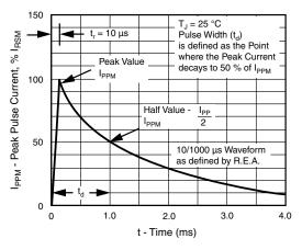
Fig. 3 - Pulse Waveform
