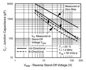
Fig. 4 - Typical Junction Capacitance
