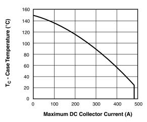
Fig. 3 - Case Temperature vs. Maximum Collector Current
