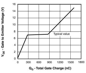
Fig. 5 - Typical Gate Charge vs. Gate to Emitter Voltage
