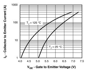
Fig. 2 - Typical Transfer Characteristics
